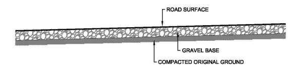
Figure 2.9 Cross-section of a typical road
