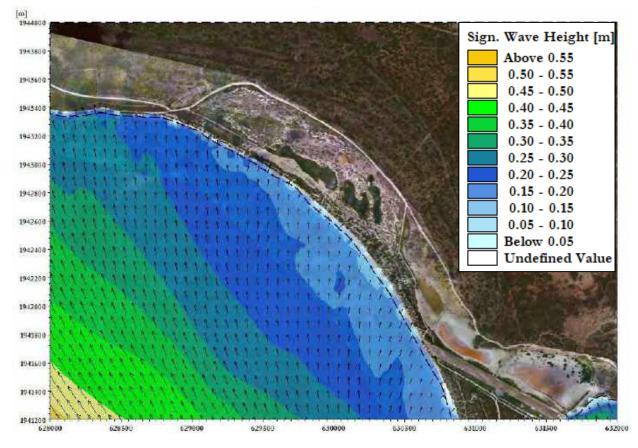
Figure 4.10 20-year mean wave heights and directions
