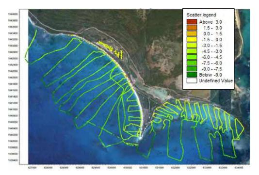
Figure 4.1 Bathymetric data points from the boat-based bathymetry survey
