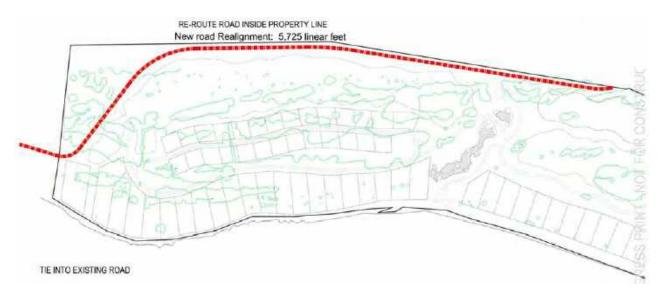
Figure 2.6 Road Realignment Phase 1
