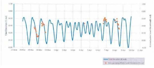
Figure 4.6 Tidal and well water level fluctuations
