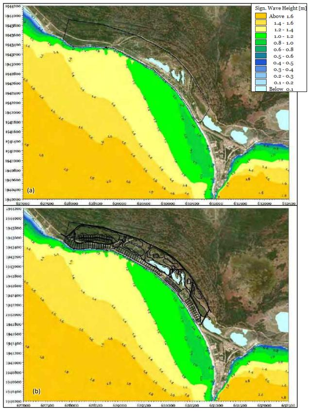
Figure 5.8 Comparison of wave heights statistically exceeded 12hrs per year (a) under existing and (b) proposed
