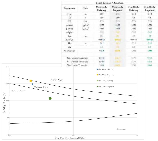
Figure 5.6 Sediment erosion and accretion zones (Ahrens & Hands); spreadsheet in inset
