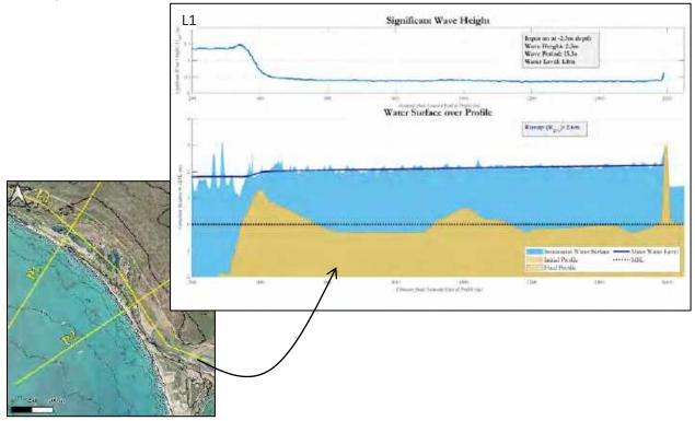
*Figure 5.5 Model results for wave run-up and wind setup at the southern boundary with the concept in place*
