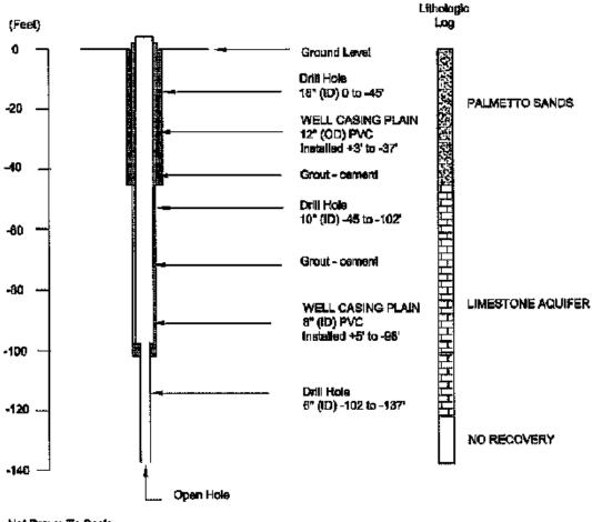
Figure 4-2: SCHEMATIC AS-BUILT DESIGN -- BRINE DISPOSAL WELL
