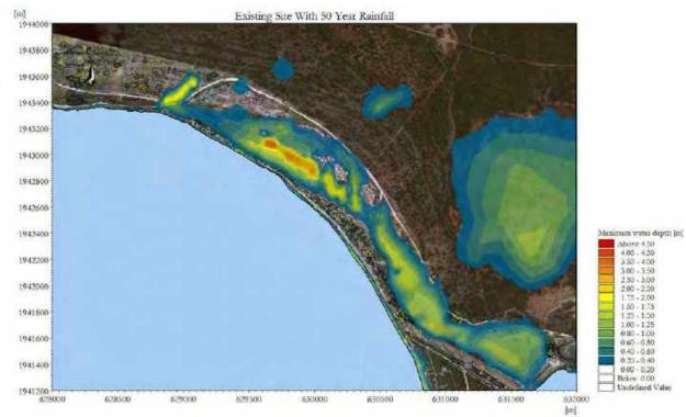
Figure 9.9 simulations using existing site with 50yr rainfall plot
