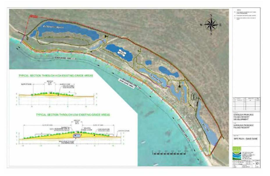
*Figure 5.4 Plan and cross-sections of proposed vegetated sand dune (shown in plan in orange)*
