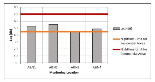
Figure 4.9 Ambient noise monitoring results & comparison to recommended nighttime limits
