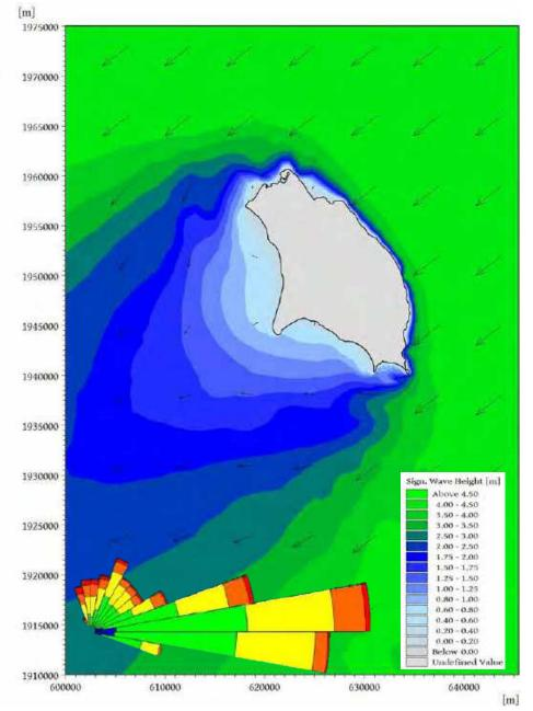
*Figure 4.8 Mean annual wave climate around Barbuda and wave rose showing the distribution of wave directions*
