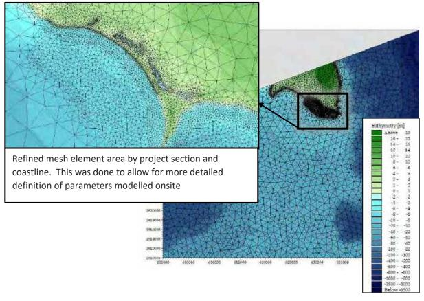
Figure 4.7 Numerical model domain - Flexible mesh used when modelling the existing conditions on the site
