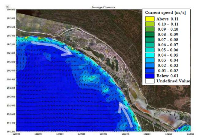
Figure 4.5 Current speeds and directions at the project site
