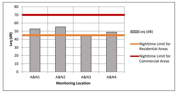
Figure 4.22 Nighttime Leq in Comparison to World Bank Noise Guidelines
