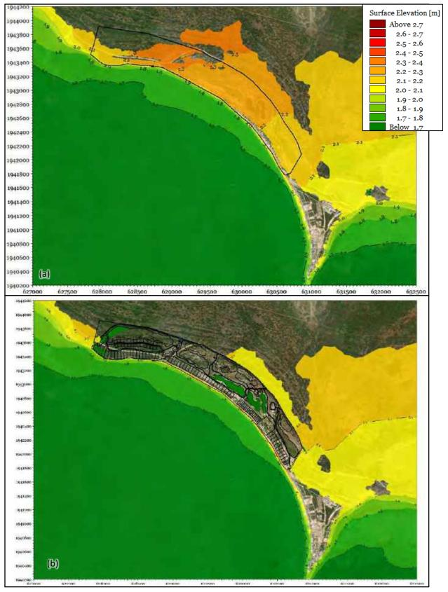
*Figure 5.12* Comparison of 50-year storm simulation results for water elevations for (a) existing and (b) proposed
