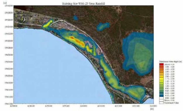
Figure 9.8 simulations using existing site with 25yr rainfall plot
