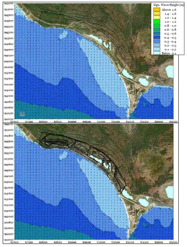
Figure 5.7 Comparison of mean annual waves results (a) under existing conditions and (b) with the plan in place
