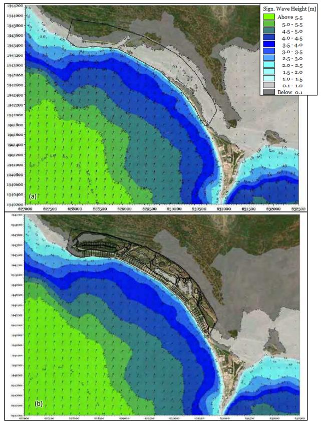
*Figure 5.14 Comparison of 50-year storm simulation results for storm waves (a) existing and (b) proposed*
