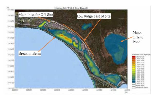
Figure 9.5 Main observations from simulations using existing site with 2yr rainfall plot
