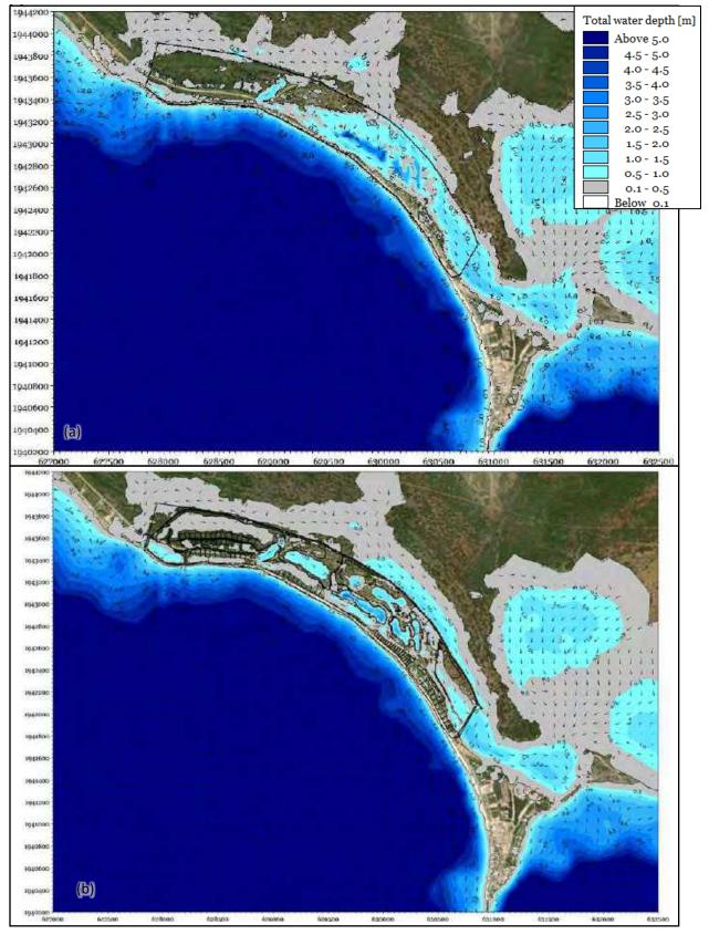
Figure 5.20 Comparison of existing and proposed drainage solutions subjected to a 50-year rainfall event
