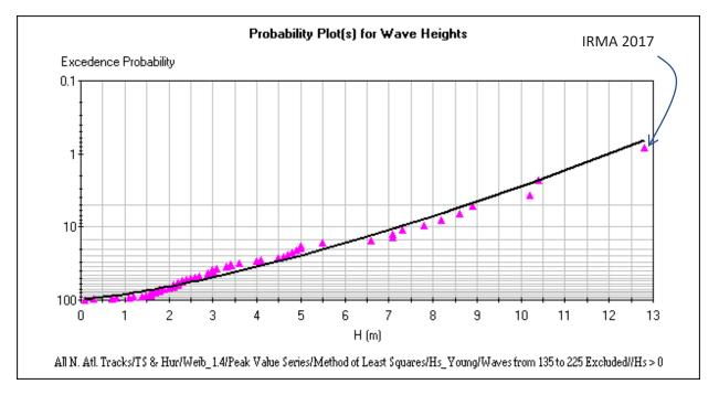
*Figure 4.14 Probability of exceedance plots for significant wave heights for past hurricane waves approaching from the south*
