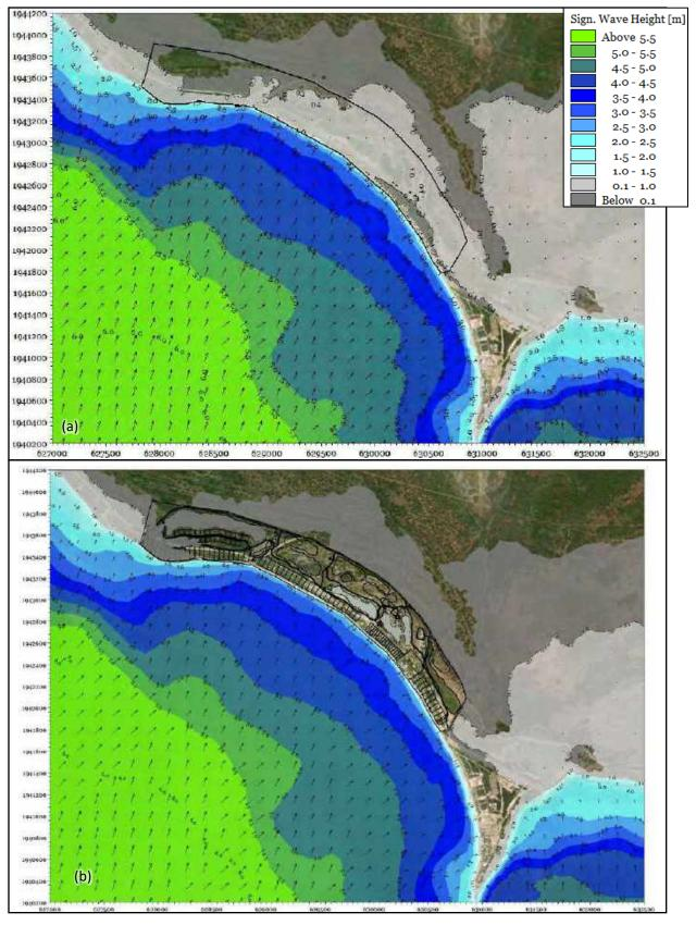
*Figure 5.15 Comparison of 100-year storm simulation results for storm waves (a) existing and (b) proposed*
