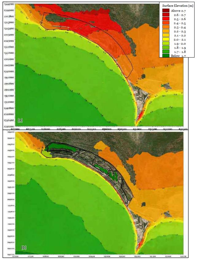
*Figure 5.13 Comparison of 100-year storm simulation results for water elevations for (a) existing and (b) proposed*
