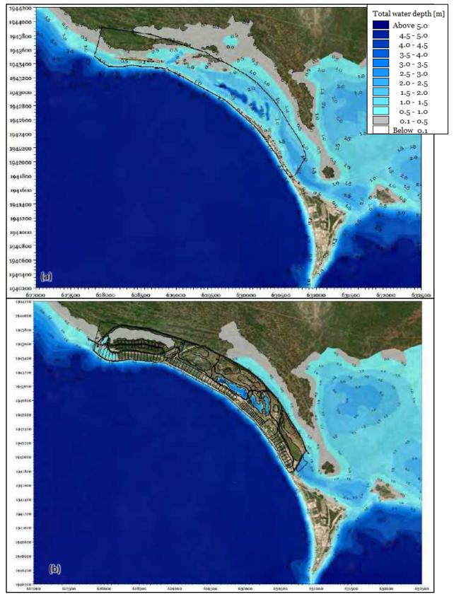
*Figure 5.11* Comparison of 100-year storm simulation results for water depths (a) under existing and (b) proposed
