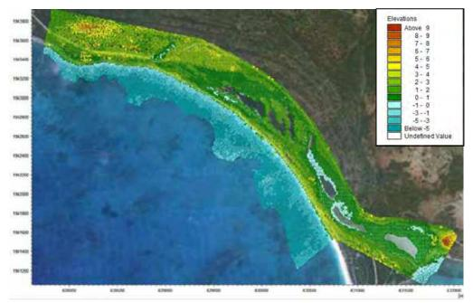
*Figure 4.2 Topographic data points from the DEM of the site and nearshore*
