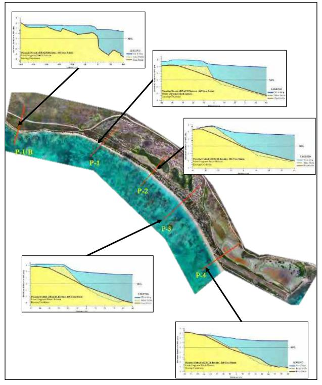
Figure 4.15 Plan with profile lines and beach erosion for a 100-year event
