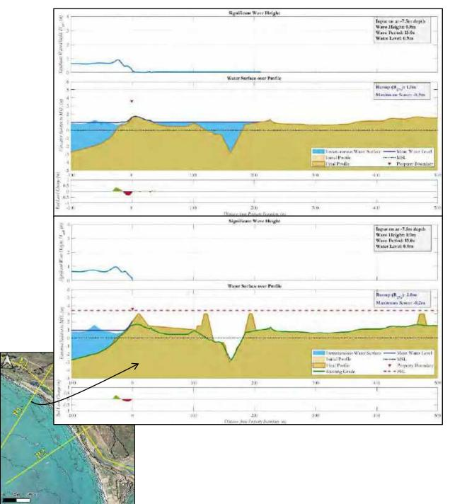
Figure 5.9 Comparison of erosion scour during 99.86th percentile wave conditions
