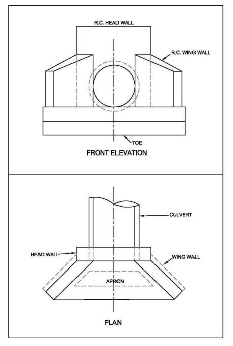
*Figure 2.12 Front elevation and plan of the end of a culvert*
