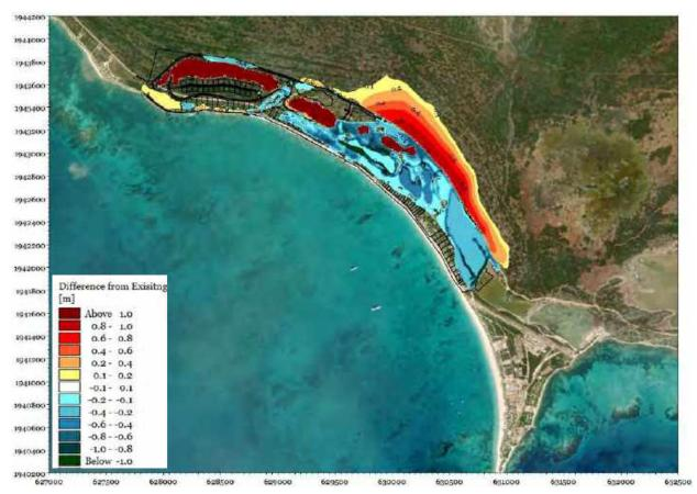
Figure 5.22 Total water depth difference plot for the 100-year event (proposed minus existing)
