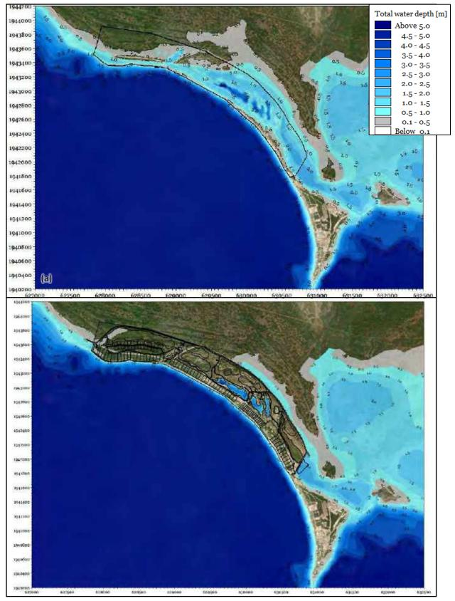
Figure 4.17 Storm surge comparison pre-development (top) and post-development (bottom) for the 50yr storm
