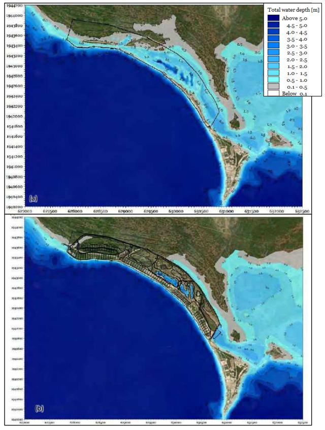
Figure 5.10 Comparison of 50-year storm simulation results for water depths (a) under existing and (b) proposed
