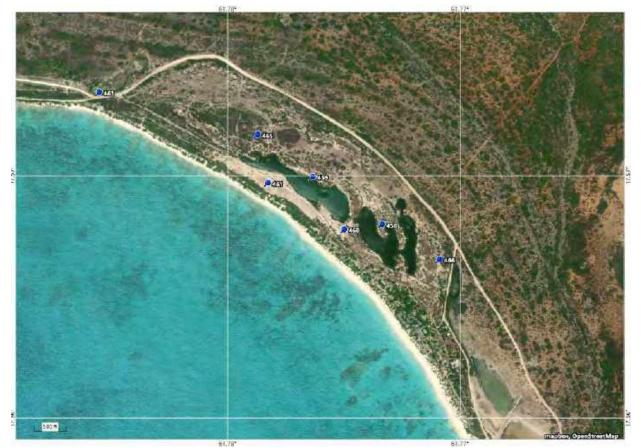
*Figure 6.9* The distribution of the water levels monitoring points across the site, established for baseline and post development monitoring
