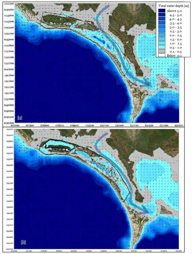
Figure 5.21 Comparison of existing and proposed drainage solutions subjected to a 100-year rainfall event
