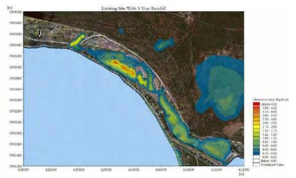
Figure 9.6 simulations using existing site with 5yr rainfall plot
