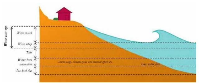
Figure 5.16 The water level components that contribute to coastal flooding
