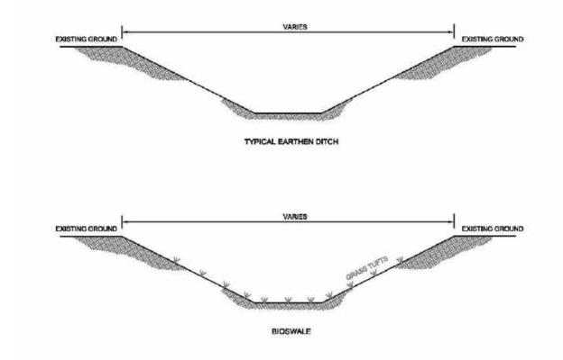
Figure 2.10 Cross-section of typical earthen ditch (top) and bioswale (bottom)
