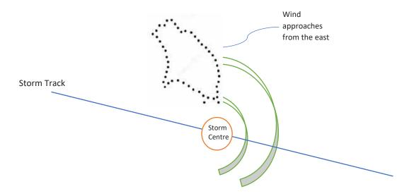
Figure 4.13 Schematic diagram of wind & wave directions from hurricane conditions
