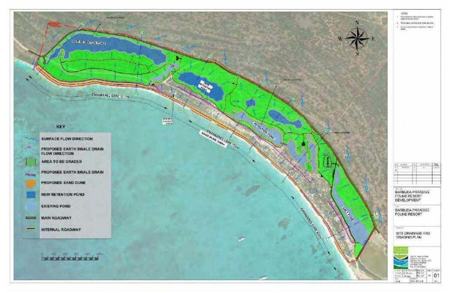
Figure 5.19 Proposed drainage plan
