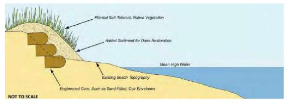
Figure 5.3 Engineered core dune<sup>15</sup>
