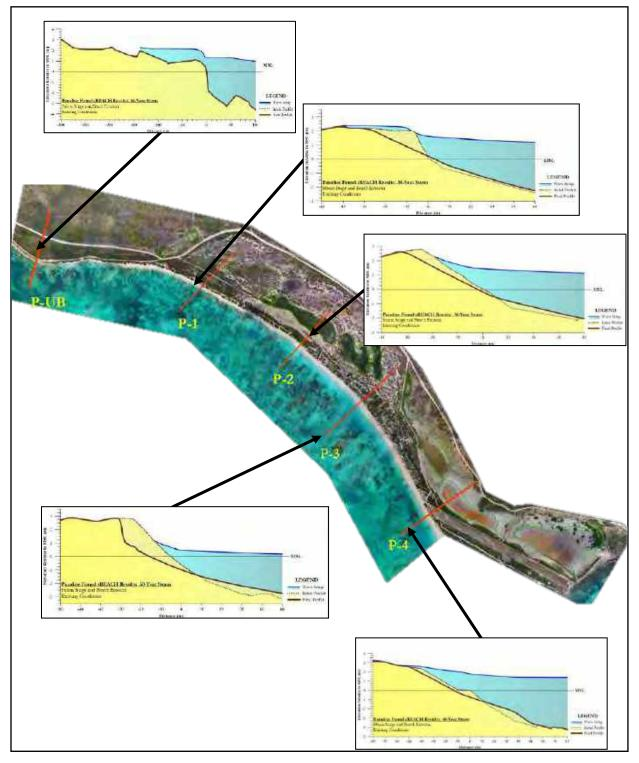
Figure 4.14 Plan with profile lines and beach erosion for a 50-year event
