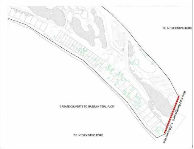
Figure 2.7 Road Realignment Phase 2
